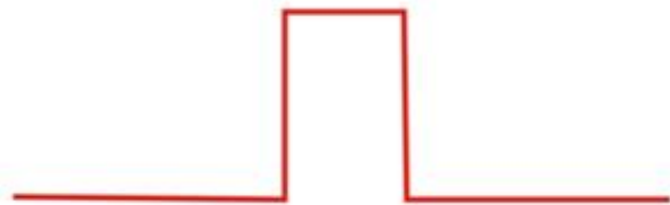
Step-index single-mode fiber
